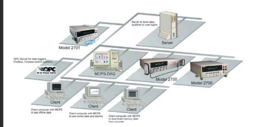
For distributed area or non-GPIB datalogging applications, the Ethernet-enabled Model 2701 supports up to 40 channels in a single enclosure and ensures simple instrumentation networking. That means the Model 2701 can be placed near the measurement process while MCPS runs on a central PC (server), minimizing noise and signal errors.
